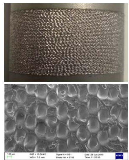
Example of laser textured stainless steel pin of (a) 10 mm diameter and (b) at high magnification
