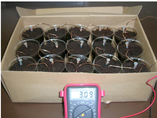
Figure 2: Bog battery. Student from the 2008-9 cohort.
