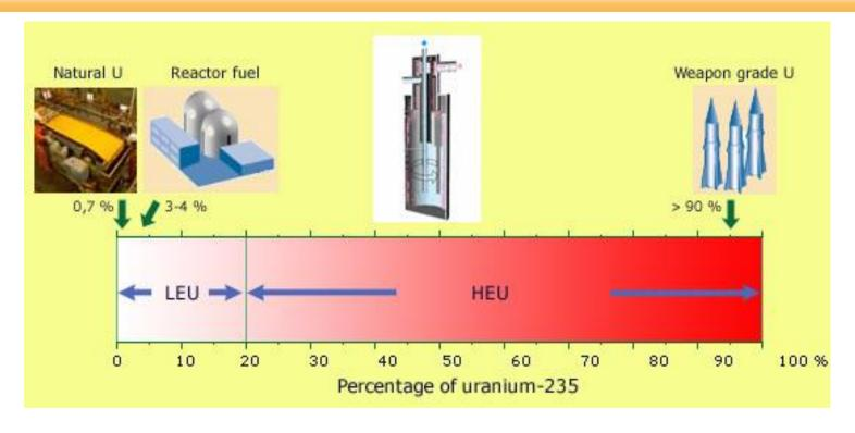
The boundary between the uranium meant for civilian uses (low-enriched uranium) and that uranium meant for military use (highly-enriched uranium) is generally fixed at 20%.
